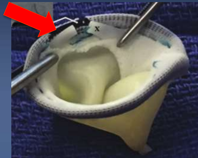
Figure 2: Fractured 21 mm Mitroflow Bioprosthesis Valve
